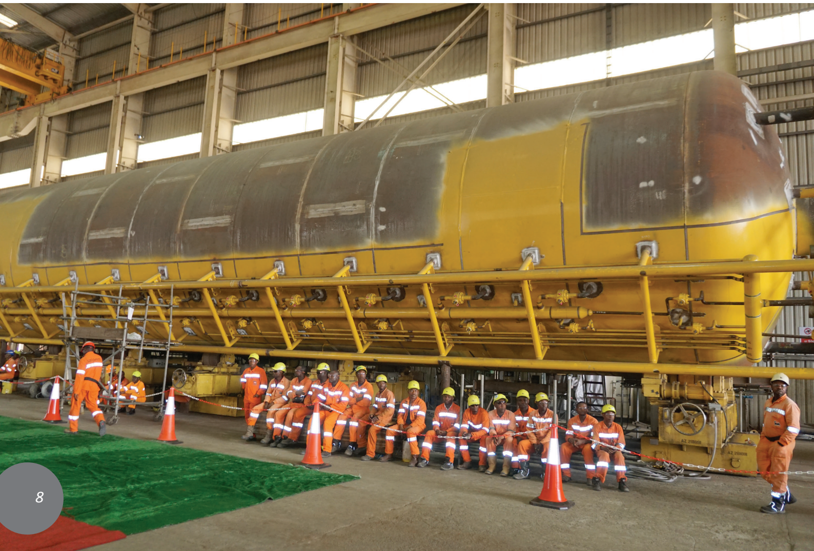
Buoyancy tank fabricated by Saipem Contracting Nigeria Limited for the Egina project
